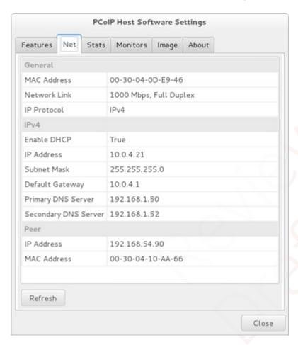
The **Net** tab shows the current network information for the host. This tab also reports status information on the NIC of the PCoIP host (speed, duplex setting, and link state—up/down). It also displays the IP and MAC addresses of the client connected to the host under the **Peer** settings.
