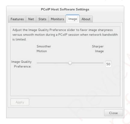
The PCoIP protocol adjusts image quality settings when the network connection between a PCoIP host and client is constrained and unable to provide enough bandwidth to support full frame rate video. The **Image Quality Preference** setting lets you configure a preference for smoother motion (higher frame rate) versus sharper image (higher image quality).
